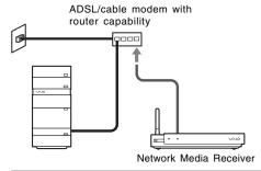
B No open LAN port available on the ADSL/cable modem with router capability
